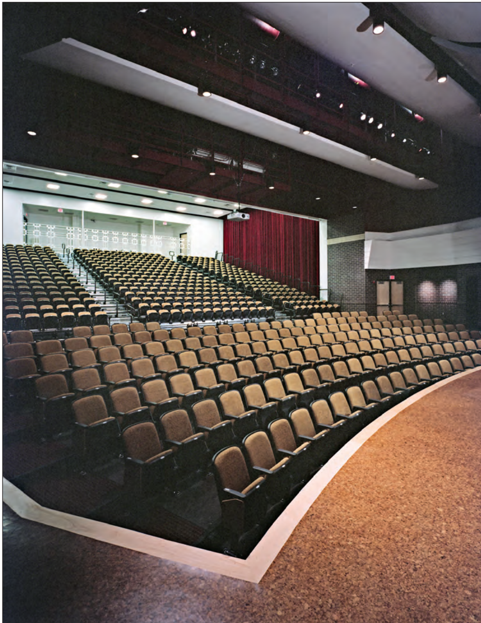
Telescoping bleachers expand backward into the cafeteria and increase the theater's seating capacity from 179 fixed seats to 663 seats.
